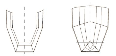
The plans provide two ways to draw and cut the bulkheads:
