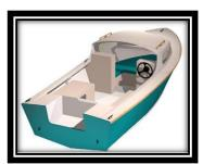
The builder is given complete freedom to adapt the cockpit layout to his preferences. The plans show all dimensions to build the boat with a wide-open cockpit and minimal framing or with benches, long or short. The cabin bulkhead can be built with one or two consoles, with a closed or open port side.
