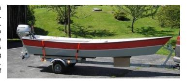
The plans include three different layouts: the cockpit style shown above, a traditional set up with three transversal benches and a full deck. The cockpit layout is very convenient: there is ample room and access under the benches for batteries, portable fuel tanks and gear. Buoyancy foam can be added to make the boat unsinkable: we specify amount and location on the plans.
