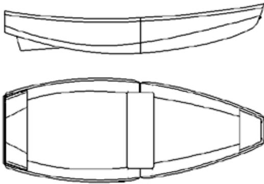
Less than 6' (1,80m) long when nested but almost 11' assembled, this dinghy is not only ideal to store on deck of a larger boat but in the back of a pickup truck or for the winter in a corner of the garage. The two parts are locked together by the removable center seat and secured by a set of simple bolts with wing nuts. She rows well but can also be fitted with the same sprit sail than the D4 and PK78. She can take up to 4 HP: the plans show transom reinforcements for outboard use.
