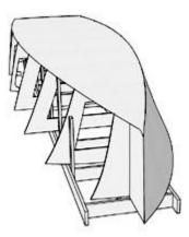
The simple flat bottom hull is easy to build and comes together fast. Only the side panel require some special attention. To create the nice flare at the bow, we use 6 slits in the panels.
