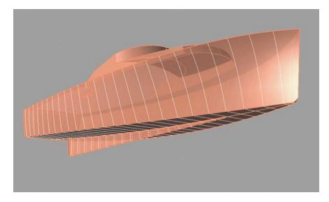
There is small amount of tumble home at the stern. There, if the builder uses Okoume, no slits are required. For stiffer plywood, we cut two slits.
