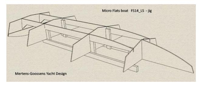
The plans show notches in the frames and stringers: no need to measure the distances on the strongbacks. The long hull panels are assembled with butt blocks or fiberglass splices (puzzle joints in the kit version). The center part of the cockpit sole is reinforced by a butt block and can take a bolted grab rail installed with marine type SS toggle bolts. The hull is unsinkable thanks to foam poured under the sole.
