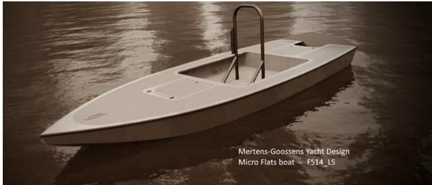
The hull is made from 6 mm Okoume plywood, epoxy, and fiberglass. The F\$14\_LS is built upside down, on a simple jig, with the hull panels planked around the frames. After the outside fiberglassing, the hull is turned over, the inside framing, stringers included, is removed and the inside is fiberglassed. The stringers and frames are installed in the fiberglassed hull. Soles and deck cover those parts.
