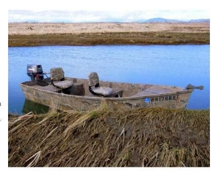
An important option is buoyancy. You can make your FS14 unsinkable by pouring two-part foam in strategic locations. The building notes suggest pouring the foam in unusable corners. The hull floats by itself: the density of our material is less than water (or plain fiberglass) but you will need foam to support the weight of the engine and the crew.
