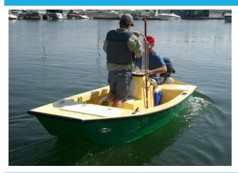
The boat is built in stitch and glue fashion but most of the hull, the bottom especially, is a true composite sandwich. The plywood bottom is sandwiched between layers of directional glass, and it is the fiberglass that supplies most of the strength, not the plywood. As in our other boats, the frames and seat tops are part of the structure.
