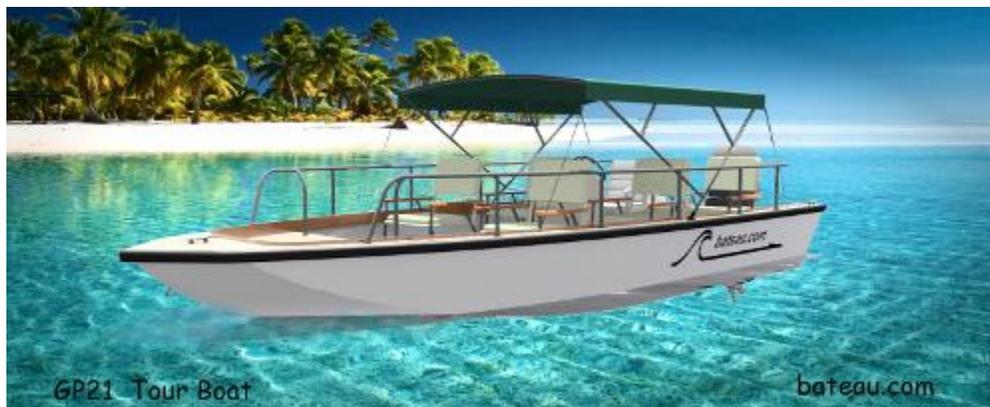
The GP21 is a wide garvey hull with good planing characteristics, stable, roomy and smooth running in a moderate chop. The hull is based on a proven work boat shape. There are several companies producing variations on that type of hull, mostly in aluminum.
