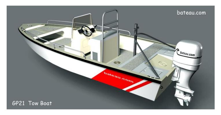
The tow/rescue boat can be fitted with a samson post (tow bar) or a swing rail bolted on the transom like the TurboSwing. The plans show specifications for a tow post bolted to the stringers and frame structure. A seat/bolster with protective backrest is also shown on the plans.
