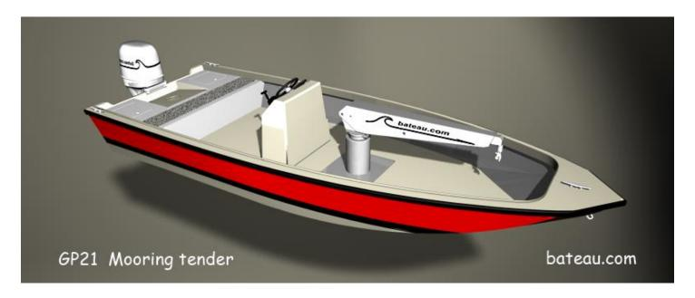
Yacht clubs and marinas will put the crane tender to good use for handling mooring, buoys and pilings. The plans show how to bolt the crane base plate to the stringers and floor frames.
