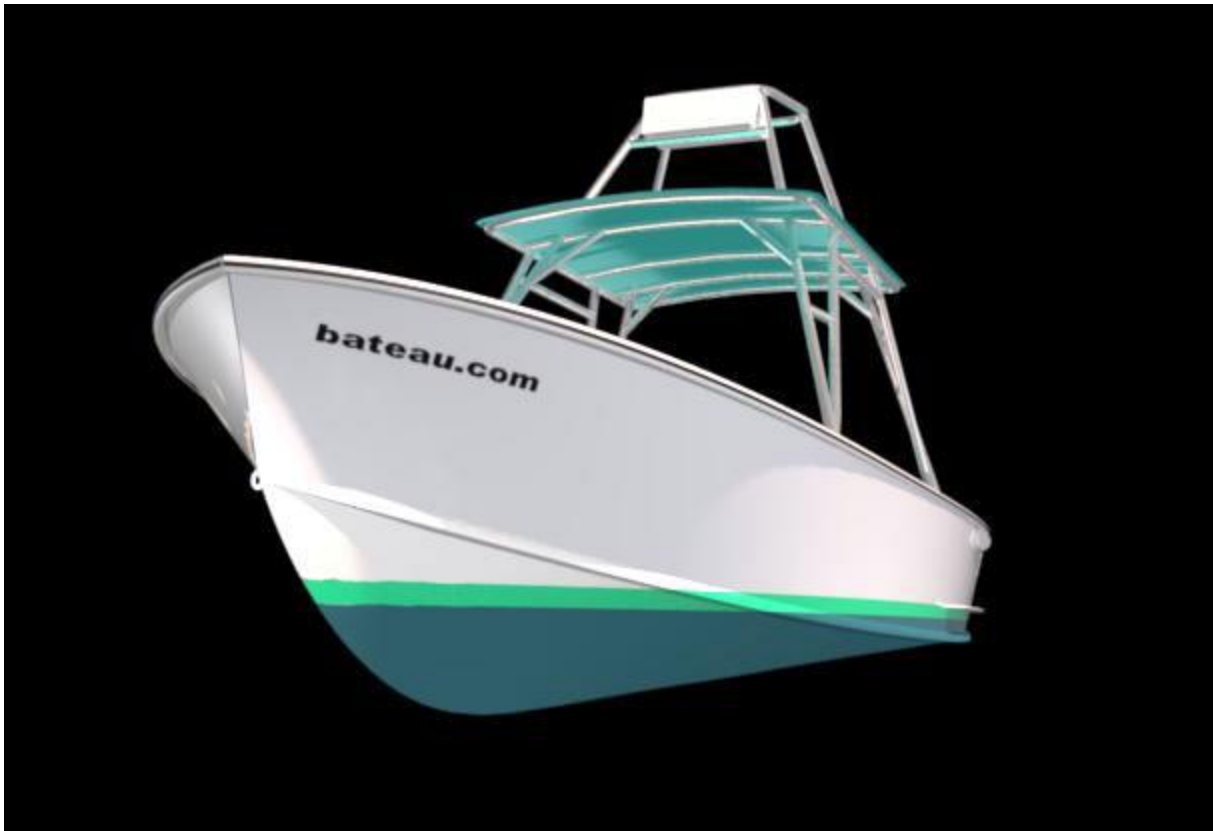
The flare in the bow is easy to create with a few slits in the side panels.
