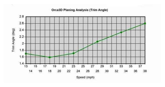
To push her over 30 mph increases trim excessively, do not install exceedingly large engines. The hull is calculated for a single 600 lbs engine on the transom. The combined weight of twin engines can not exceed 800 lbs.
