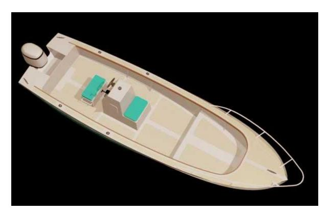
The plans show a classic layout with casting deck and center console. The cockpit is almost  $21' \log (6,30m)$  and more than 28'' deep (72 cm) at its lowest point.
