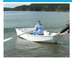
This boat is built in stitch and glue, from flat plywood panels assembled with epoxy-fiberglass tape. For a detailed description of the stitch and glue boat building method, see our "How To" section where you will find a complete illustrated tutorial as well as information about epoxy, fiberglass and plywood.
