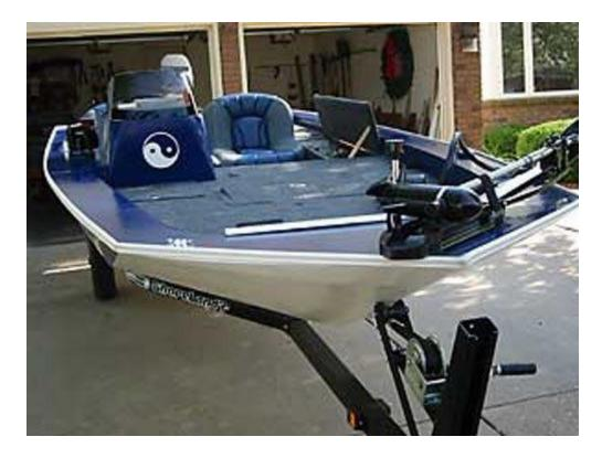
The program of the boat is clear: a comfortable, roomy and stable platform for family outings or fishing in protected waters. While the vee hull can take a nasty chop at high speed, she does not have enough freeboard for offshore use.
