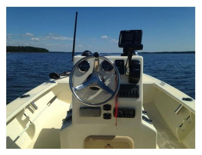
The cockpit is self bailing: even with a heavy load, the sole stays well above the waterline, an unusual feature in a boat of this size.
