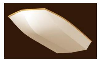
Our boat has a cleaner and more efficient hull shape than the Boston Whaler®: a true vee hull with chines almost straight in plan view and a wide deck. It shows a good combination of stability with a roomy deck on a vee hull that will run much smoother than a Carolina Skiff®.
