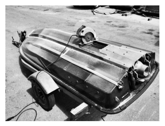
The builder will cut the almost complete fiberglass bottom out of a jet ski, jet pump and motor included, cut and opening in our plywood composite hull and drop the jet ski assembly in the JA18.
