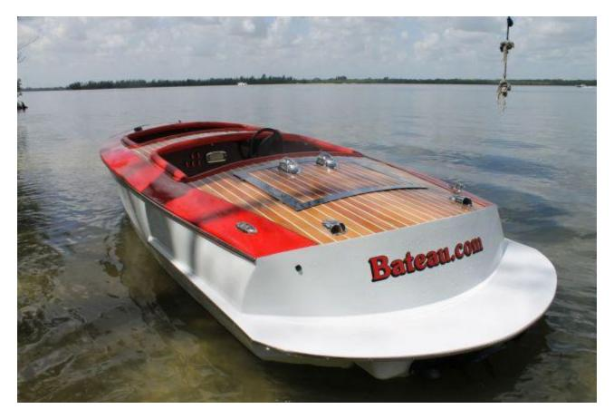
Calculated hull weight is 580 lbs for a complete hull, all plywood, glass, epoxy, paint ready to be rigged with the jet engine.
