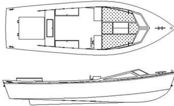
A small traditional lobster boat that can be used as a fishing launch or picnic boat. Economical and versatile semi-displacement hull.
