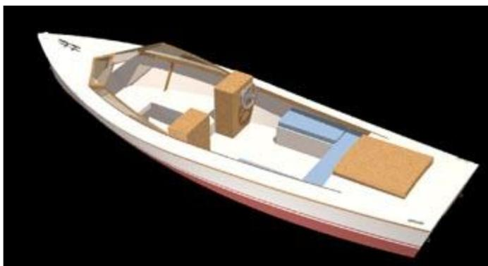
The hull can be built the stitch and glue way, upright with panels folded around the frames or better upside down, using the frames as a jig. See the [our building tutorial for a step by step overview](#) of the process.
