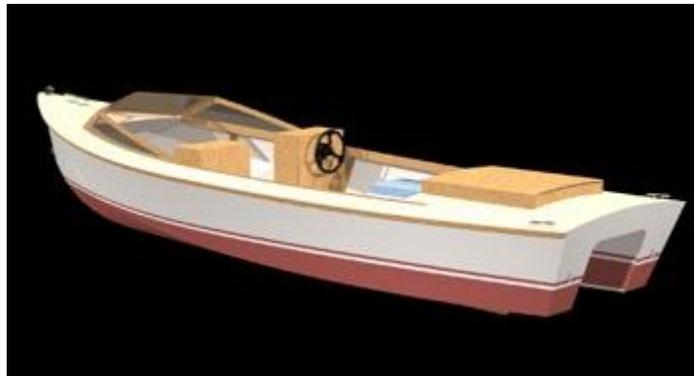
Lobster boats, picnic launches and many large sport fishing boats are variations on the double wedge hull shape. Those boats go fast with little power, not as fast as planing hulls (monohedron type) but they keep going at the same steady speed when the planing hulls are forced to slow down. Do a search on the Internet to read more praise about this type of hull.
