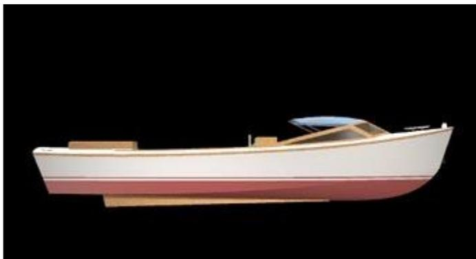
While our fiberglass/plywood composite material is 100% original, there isn't anything new in the hull lines. It is a proven type with very predictable behavior. For the looks and layout, we took ideas from several classic designs: the cuddy cabin is inspired by the Atkins design Ninigret, the open version windshield comes from Bolger's Halloween, the engine cover from the Handy Billy that was featured in Wooden Boats. We mixed it all with a touch of Culler's influence and it became the Nina.
