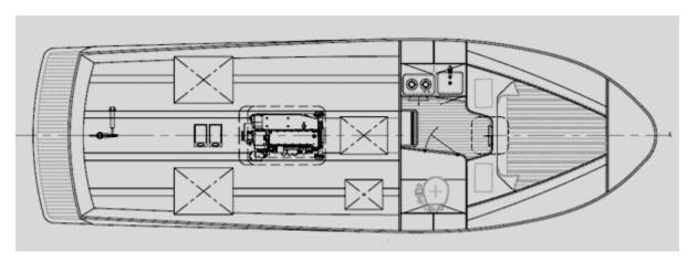
There is standing headroom where needed, under the open companionway in front of the galley. Headroom in the head is max. 5'(1,50 m), sitting headroom is a comfortable 4'(1,15 m).
