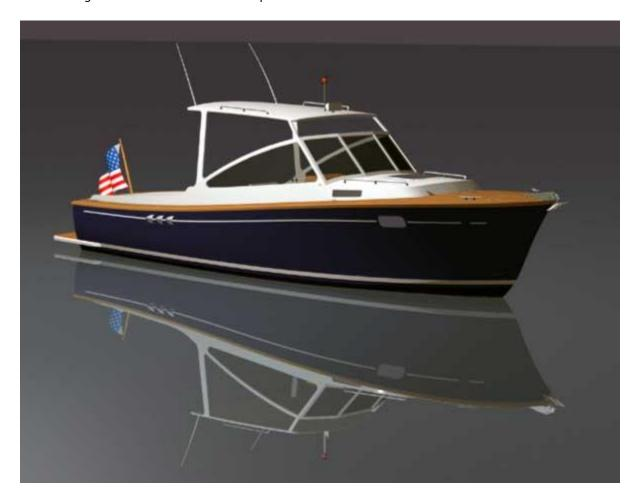
The plans can be customized as long as the builder does not compromise the structure. Seating can added to the cockpit, the cabin layout can be changed, the hard top can be different but the cabin height should not be increased excessively and if the boat is fitted with a pilot house, it must be kept very light.
