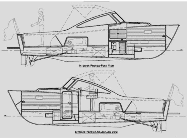
An anchor locker is located forward of the collision bulkhead. There is plenty of storage under the vee berth, in the cockpit under the gunwales and in the transom.
