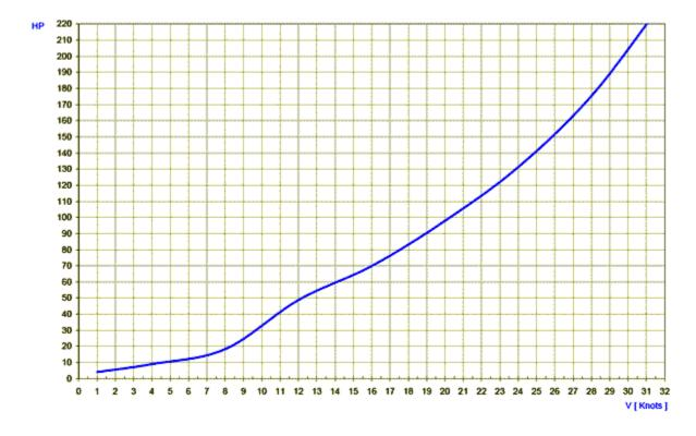
Above is the speed/HP curve calculated per Savistky-Koelbel for the LB26 at 2.450 Kg fitted with a Nanni Diesel 390 TDI 200 Hp. This shows a nice cruising speed of 25 mph (21.7 knots) using 110 HP and a top speed of more than 30
