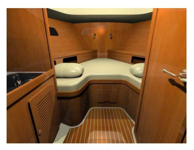
Inside there is a roomy cabin with vee berths 2 meters long (79"), a small but practical galley on the port side and a fully enclosed head on starboard. Freshwater and waste tanks are 26 gallons (105 liters) each and there is room for more.
