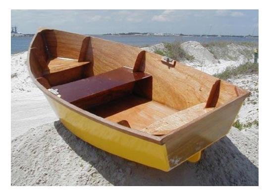
**Required Skills:** The Nutshell is very easy and fast to build, there are no butt joints. The sides are cut from one standard sheet of plywood.
