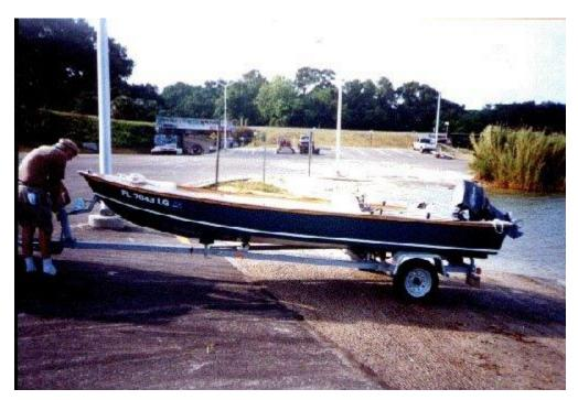
This boats transom is designed for a standard 15" shaft. The transom can easily be modified to accept other shaft lengths.
