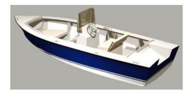
All the plywood parts have been precisely calculated: you cut them flat on the floor, no need for templates, no need to take measurements from the hull framing as in the plywood on frame method.
