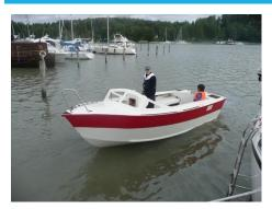
The hull is identical to the C17 design: generous volume, ample freeboard, well defended bow. In proper hands, this boat can take bad weather safely. The deadrise is 45 degrees at the cutwater progressing towards 11 degrees at the transom. This is an ideal hull shape that will run smoothly in bad weather but with a vee moderate enough to provide good stability at slow speed without the wild roll typical of deeper vee hulls.
