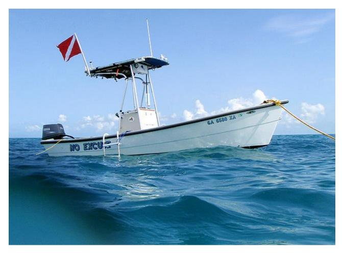
The OD18 is the big brother of the OD16. The OD16 was first designed as an 18' hull then shrunk in length to 16' at the request of the first builder. The OD18 hull is longer but has the same beam and freeboard. Each boat, OD16 or OD18, has the slanted chine.
