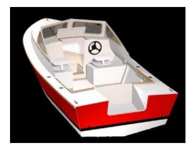
The self bailing cockpit depth minimum 26" with 12" wide gunwales, is another important element of safety. Her PPI is at DWL is 543 lbs (247 kg). Thanks to the freeboard and transom design, she can be rated to a max. capacity of eight persons (USCG) and we recommend engines in the 90 to 150 HP range. While stronger than the typical production fiberglass boat of that size, she is also lighter and does not require as much HP (or fuel) to cruise at the same speed.
