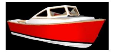
The generous freeboard and the classic sheer are tried and true features contributing to seaworthiness. This boat will negotiate both head and following seas with ease. Lightly loaded, the P21 will require 90 HP to cruise in the low 30 mph range. 125 HP is recommended for a well equipped boat at full load.
