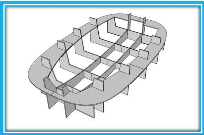
The **Club Racer** can be built two ways. The first is with the use of a basket mold system. A basket mold has the advantage of tighter tolerances and much faster production of multiple hulls. The basket mold system for the **Club Racer** is sold separately [and can be found here](#), it is a great solution for a club or organization that would like to build a number of boats. The design of our basket mold is copyrighted.
