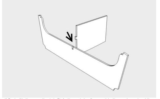
Once you are satisfied with the way the tab fits in the notch, disassemble the parts and put them aside.
