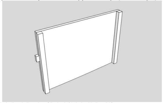
Epoxy glue the battens to the edge of the trunk side but not to the mid frame. Epoxy glue the other side of the trunk to the cleats to form a box.
