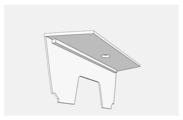
The partner sits on top of the frame. Edges are flush. The two parts are epoxy glued with a corner cleat. The section of the cleat is unimportant: 1" square is fine or use leftover plywood as for the trunk. Note that the cleat does extend all the way to the sides.
