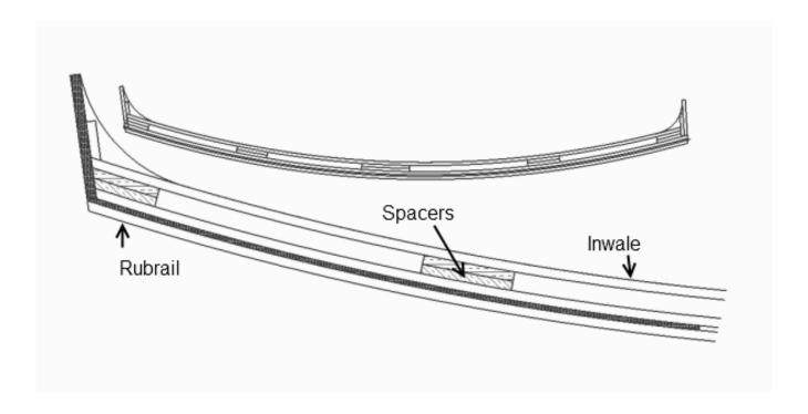
The coaming itself is a long piece of plywood that cover the edge of the side panel. It is glued on top of the rubrail, inwale and spacers.
