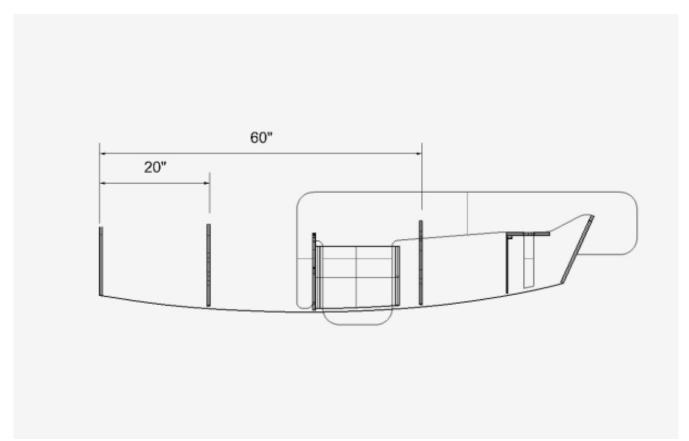
The locator grabs the bow stern and the mid frame, it also goes through the dagger board trunk
