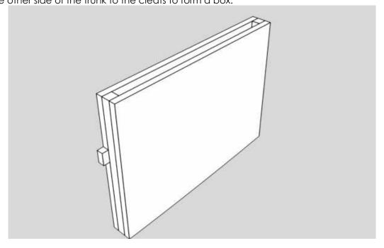
(Before assembly, all faces of the trunk must be coated with epoxy.)
