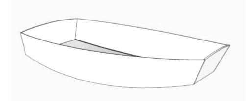
The sides and bottom are joined by loose stitches and barely touch at their edges. A 1/4" space is ideal, we will tighten the stitches later. (The stitching procedure is explained in our "Stitch and Glue 101" tutorial.) The two transoms are located between the sides and bottom. We use temporary screws (dry wall screws are perfect) to hold them together. As for the stitches, do not tighten the screws, screw them in just enough to have contact between the parts.
