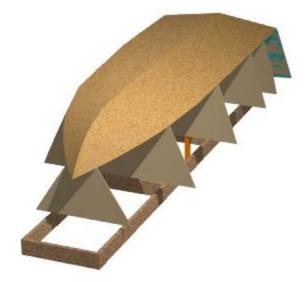
Our jig system is very uncomplicated, self-aligning and economical since we use the internal framing of the hull as molds. Our jig does not require all the precautions, alignments or even a perfectly flat floor that are a must for traditional boat building.
