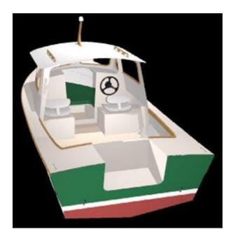
The self bailing cockpit depth minimum 26" with 12" wide gunwales, is another important element of safety. Thanks to the freeboard and transom design, she can be rated to a max. capacity of eight persons (USCG) and we recommend engines in the 90 to 125 HP range. While stronger than the typical production fiberglass boat of that size, she is also lighter and does not require as much HP (or fuel) to cruise at the same speed.
