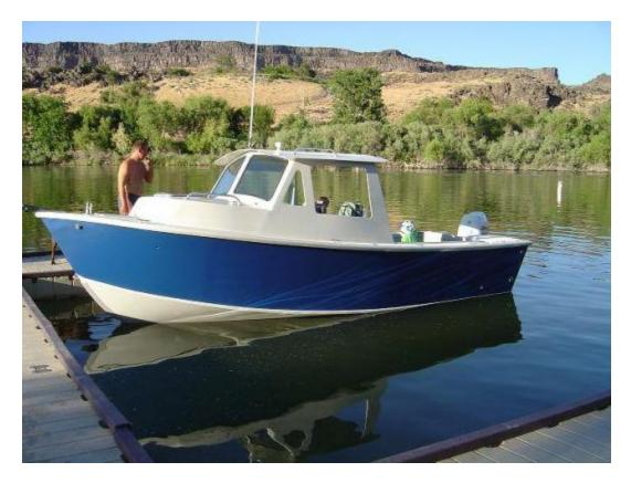
The generous freeboard and the classic sheer are tried and true features contributing to seaworthiness. This boat will negotiate both head and following seas with ease. Lightly loaded, the P21 will require 90 HP to cruise in the low 30 mph range. 125 HP is recommended for a well equipped boat at full load.
