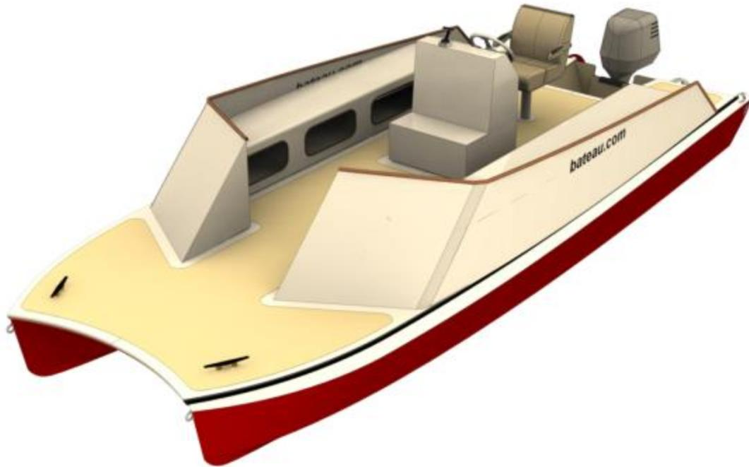
The fine hulls allow this boat to move relatively fast with a small outboard, much faster than a monohull of the same length. With a larger engine, the boat will get on plane without having to push through a steep bow wave: the boat is comfortable at any speed in between. Compared to cylindrical pontoons, the asymmetrical catamaran hulls result in a better water flow between the hulls with less restrictions or wasteful turbulence.
