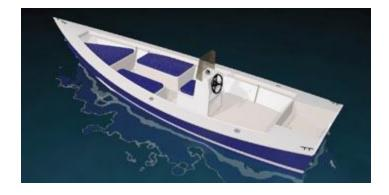
The builder is given complete freedom in the layout of the boat. As long as the frames shown on the plans are present and common sense is used in weight distribution, almost anything is possible: simple open plan with a center console, thwarts, longitudinal benches, small or large casting deck etc.
