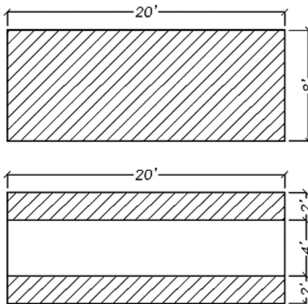
You can see that the catamaran hull as less foot print than the monohull: at equal draft, the cat displaces only half the water of the mono hull and therefore, at equal boat weight will have two times more draft.
