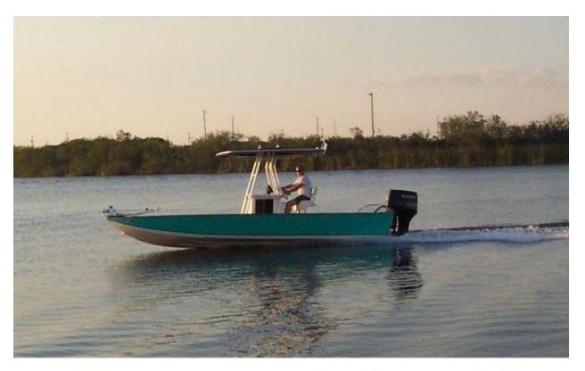
The Phantom 22 is a bay boat based on our Phantoms 16 and 18. They share the same shallow draft and hull shape but the 22' hull offers more freeboard, comfort and capability.
