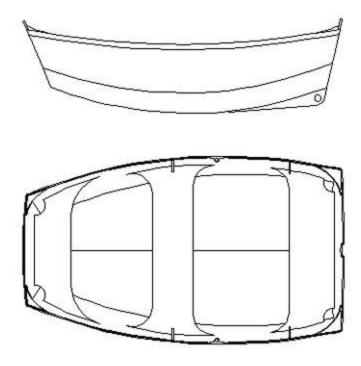
A successor to the D4. The best use of two sheets of 1/4" plywood for the hull gave us a length of almost 8' and a beam of 4' 8". She has more rocker in the bottom than the D4, is more stable thanks to her wider beam and uses a simple Optimist type (sprit) rig. The 6' or 6-1/2' oars store inboard while using the sails or the small outboard: max. 3 HP.
