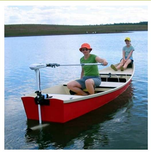
The Swift is an outboard powered square stern canoe. The fine hull will travel fast with little HP. In displacement mode, the Swift will go much faster than a wider boat. She moves with less fuss and creates only a small wake.
