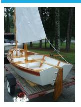
The SD11 hull is very easy to build thanks to her flat bottom. There are no plywood scarfs: we use very simple butt blocks.
