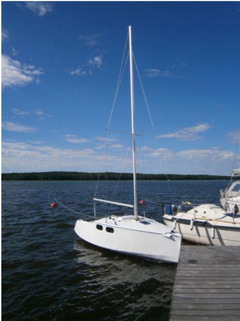
Thanks to its large battened main, the VG18 can be sailed as a catboat but she will show her full potential with the jib or spinnaker rigged on a retractable pole.
