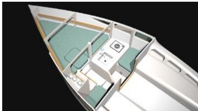
The saloon is short because priority was given to cockpit space but two long bunks (7' 8") extend under the cockpit seats.
