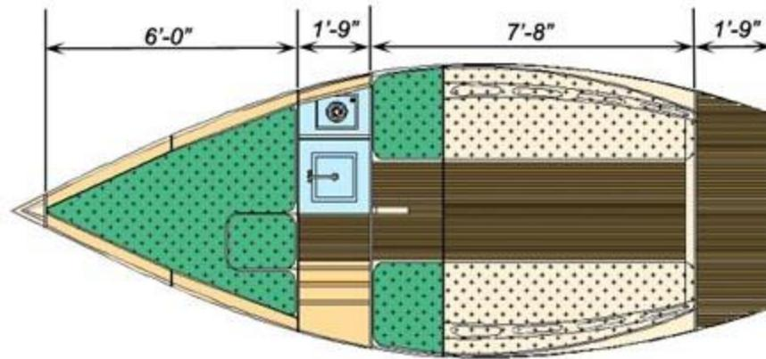
From the bow: a classic vee birth close to 7' long in diagonal with room for a Porta-Potty underneath. Immediately behind the mast bulkhead is a small galley to starboard faced by a hanging locker or storage bin to port.
