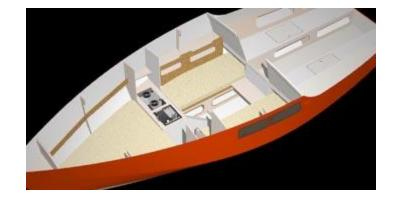
The VG23 is powered by an outboard on the transom. The outboard can be clamped directly on the transom or on a standard outboard bracket.
