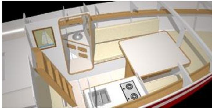
As an option, the plans show a full bulkhead behind the head and a wide cockpit seat hatch. This creates a wet locker. For that option, we show a sole in the locker, above the water line.
