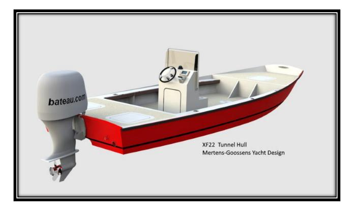
The XF22 is the big brother of our XF20: a very shallow draft tunnel hull designed specifically for fishing the flats without any compromise. Hence the name Extreme Flats 22.
