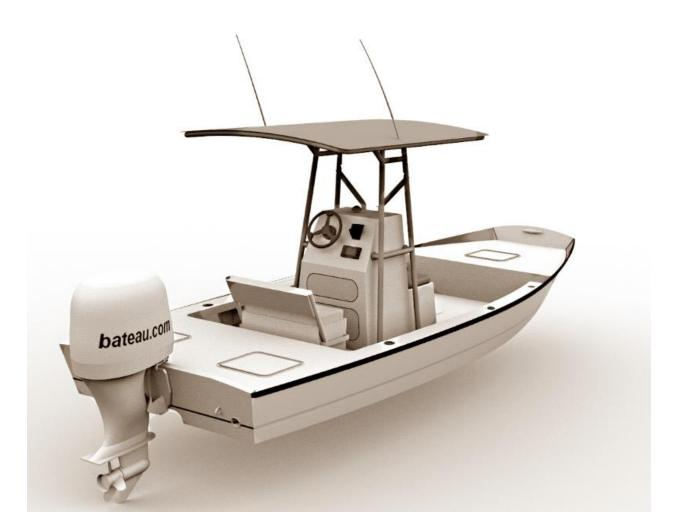
The layout of the XF22 can be adjusted to the builder's preference. The plans show two different center consoles, a standard one and a very large on as in the picture above. Casting deck and aft deck can be larger or smaller.
