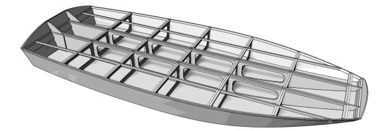
The plans show dimensions for molds to set up on strong backs, all lined up, with notches in stringers, molds and frames. This allows for a very easy set up with minimal measurements. All molds sit directly on the strongbacks, the stringers fit in notches and set the spacing. The side panels are supported by a notch on the molds. The plans show all dimensions for those parts.
