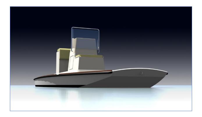
The Texas Scooter is a specialized version of our XF20: a shallow draft tunnel hull with a very low freeboard designed specifically for fishing extended flats such as those found along the coast of Texas
