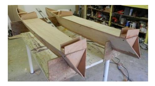
The beams simply slot into the main hull and are joined on the boat's centreline. They are normally permanently attached to each outrigger, but can be unbolted for long term storage. So it is still a fast setup, especially as the dinghy skiff style mast can be left up even with the outriggers removed. Very useful if keeping the boat in a dinghy park or storage area. A jib and a screecher are options.
