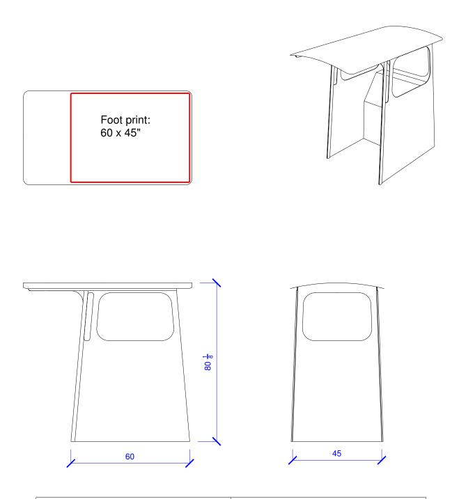
All panels from 10 mm plywood<br/>except roof = 6 mm.BOM:Seams taped with 1 layer 12 oz. biaxial<br/>outside, 2 layers inside,<br/>offset edges 1".- 5 sheets plywood 10 mm<br/>- 1 sheets plywood 6 mm<br/>- 1.5 gallon epoxy resinOutside fiberglassed with 6 oz. woven.<br/>Epoxy resin only, no polyester or glue.<br/>All surfaces inside and outside coated with<br/>epoxy resin.- 10 yards woven glass 6 oz. 50" wide.
