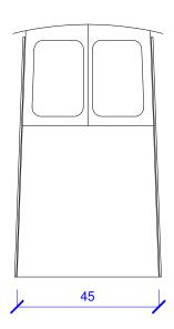
All panels from 10 mm plywood except roof = 6 mm. Seams taped with 1 layer 12 oz. biaxial outside, 2 layers inside, offset edges 1".
