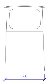
All panels from 10 mm plywood except roof = 6 mm. Seams taped with 1 layer 12 oz. biaxial outside, 2 layers inside, offset edges 1". Outside fiberglassed with 6 oz. woven.
